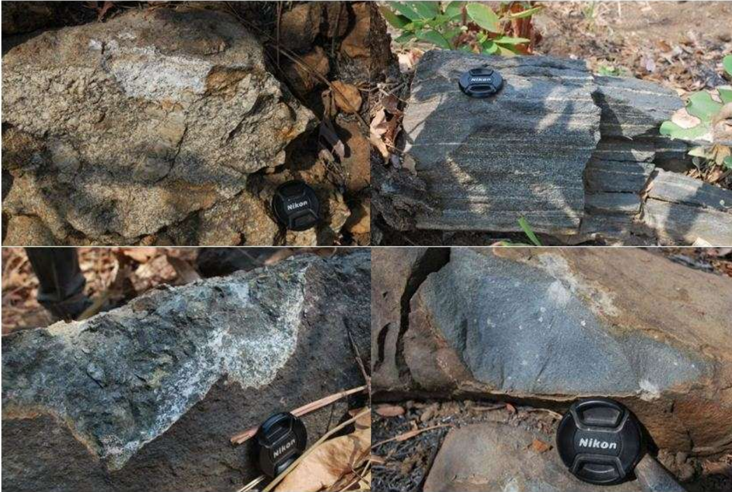
Figure: a) Coarse-grained granite with a weak foliation. b) Strongly foliation biotite-gneiss. c) Pyroxene rich, gabbroic-textured rock (at back). d) Fine-grained basalt with sulphide minerals.
