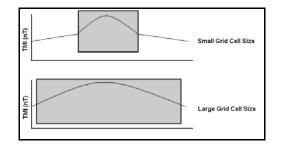
Figure 1: The scale of interpretation needs to be taken into consideration. When a small grid cell size is chosen, higher frequency anomalies will be resolved, while a coarser grid cell size will smooth high frequency noise, and only low frequency signals are resolved.
