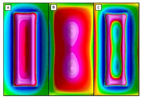
Figure3: Plots of Total Magnetic Intensity. A) Original TMI dataset gridded at 100m B) Regional TMI dataset gridded at 1km C) Residual TMI dataset produced by the subtraction of B) from A).
