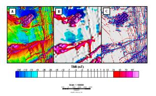
Figure 4: Plots of total magnetic field from Iroquois Falls region. A) Original TMI dataset gridded at 20m. B) Regional TMI dataset gridded at 640m. C) Residual TMI dataset produced by the subtraction of B) from A).
