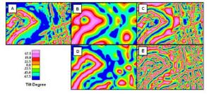
Figure 5: Tilt-Angle applied to varying grid cell sizes and depth slices of the Iroquois Falls dataset. A) Original TMI dataset gridded at 20m. B) Regional TMI dataset gridded at 640m. C) Residual TMI dataset produced by the subtraction of A) from B). D) Regional TMI dataset gridded at 320m. E) Residual TMI dataset produced by the subtraction of D) from A).
