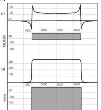
Figure 2. Cross-sections of the same rectangular prism, but with a depth to bottom of 60m (top) and the other with a depth to bottom of 20km, to approximate infinite (bottom). This plot displays the interference between the top and bottom of the source body on the resultant TMI signal.
