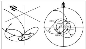
**Figure 4.** Diagrammatic representation of how the magnetic inclination of the remanence vector  $(D=210^\circ, I=60^\circ)$  measured in an individual borehole is a direct function of the orientation and inclination of each borehole relative the true magnetic vector. Intersecting the same remanence component with a number of boreholes that have different trajectories provides a determination of the true magnetic vector.
