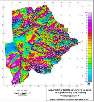
Figure 2. Total magnetic intensity after IGRF correction for the Botswana Tie Line Survey.
