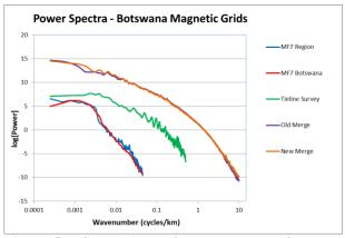
Figure 5. Comparison of power spectra for TMI grids of satellite magnetic data (CHAMP model MF7), the Tie Line Survey, and previous and new merges.
