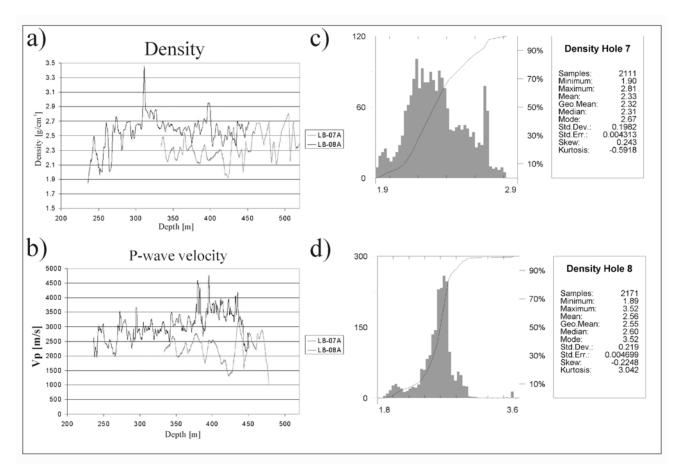
Fig. 3. Density (a) and P-wave velocity (b) profiles obtained from core scanning and borehole logging respectively. c) and d) are histograms of the density measurements done on the core obtained from Lake Bosumtwi. The median values of 2.3 g/cm<sup>3</sup> for LB-07A and 2.6 g/cm<sup>3</sup> for LB-08A are the values used in the gravity model.
