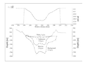
Fig. 4. A 2.5-D model of the structure based on gravity data. Observed gravity anomaly (solid curve) and calculated result (dashed curve). Vertical exaggeration is 10× (modified from Danuor 2004).
