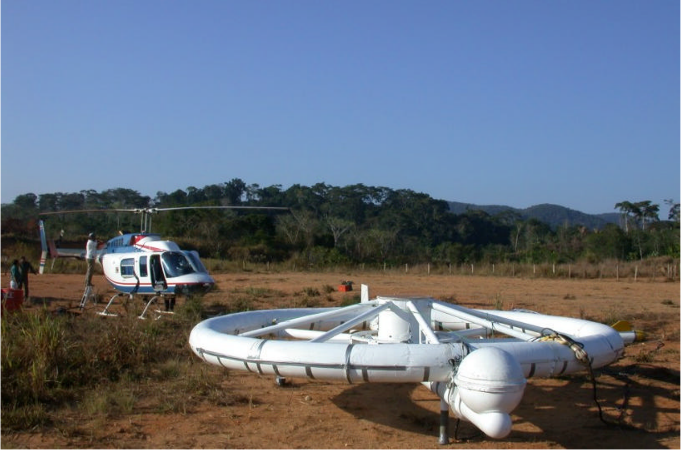
Figure 1. The AeroTEM system transmitter-receiver coils are shown here during a break in a diamond exploration program in Venezuela.
